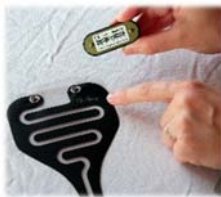
4. Fix the transmitter on the urine-detector. The polarity does not matter
