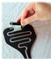
4. Fix the transmitter on the urine-detector. The polarity does not matter
